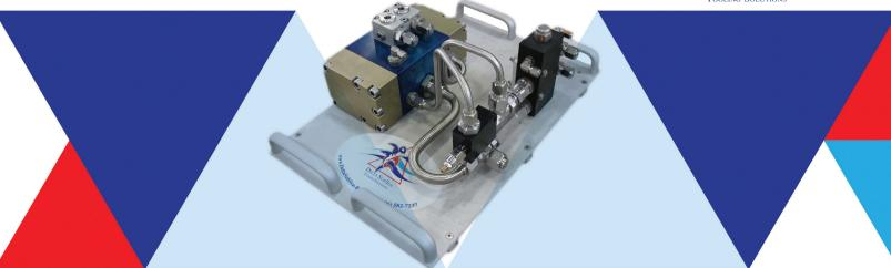
The Delta SubSea High Pressure i-HPU utilizes hydraulic energy from the ROV tooling circuit to power a reciprocating pump with a differential ratio of 1.26:1. Net differential pressure across the reciprocating pump produces an outlet pressure 1.26 times greater. Thus a 2400 psi input will provide 3000 psi output. The flow is divided by the differential ratio, thus with an input flow from the ROV of 8.8 gpm, the output from the i-HPU will be 7 gpm.
